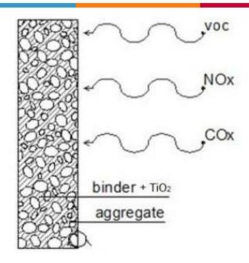
Multifunctional mortar with low environmental impact, able to improve the air quality in confined spaces, thanks to its depolluting properties, hygroscopic buffer capabilities, electromagnetic shield properties, in addition to the conventional mechanical strength and permeability properties.
