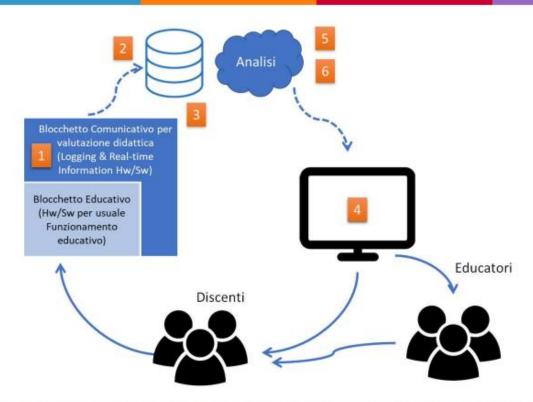
The patent consists of independent functional blocks (made up of hardware and / or software) used in Educational Robotics courses, containing algorithms capable of tracking the construction sequences implemented by the student during the execution of a task assigned to him by the teacher.
