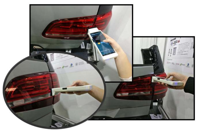
The device is integrated in a smartphone and is able to recognizes the measurement area through a Deep Learning approach. The device allows measurements to be made even on surfaces and materials that have different optical responses, as, for example: metal, plastic, chromed components, etc.
