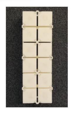
The invention consists of a metastructure designed to ensure vibration isolation over a wide frequency range. This metrastructure is a periodic structure which, thanks to the wide bandgap that characterizes it, that is the frequency range where the propagation of elastic / acoustic waves is inhibited, can be used in numerous applications where the ability to isolate vibrations is required.
