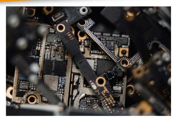
The invention concerns a new biotechnological method for recovering copper from end-of-life printed circuit boards. The process can be performed as one or a combination of two procedures, one with multi-step leaching and one with column leaching, allowing high leaching yields to be achieved with increasing concentrations of printed circuit boards (PCBs) in solution.
